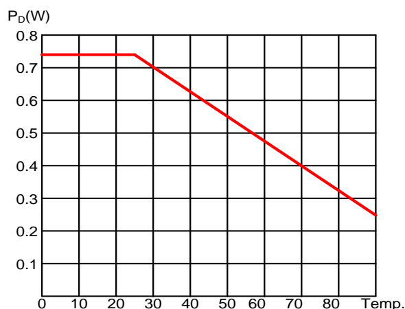
Figure 1: De-rating curve with ambient temperature on the maximum power dissipation allowed.
